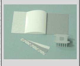
OC-7300 Spec01 is a thermally conductive phase change material having a softening temperature of  $55^{\circ}$ C. The liquid phase of the material can fill interface irregularities with much higher efficiency than traditional gap filler. On the other hand, it is a solid at room temperature and can be handled easily during installation.
