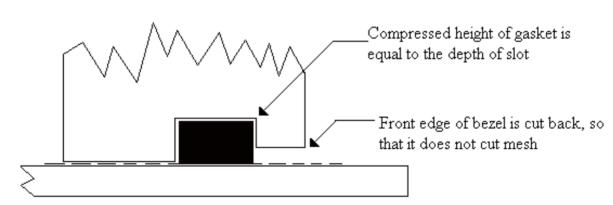
The rear surface of the front panel must be free of paint and should have a conductive plating applied for mesh contact
