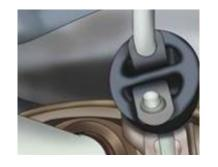
The SEM SP exhaust hanger band insert is a 100% polyester, spiral wound product that is easily molded into your exhaust hanger that gives superior performance in minimizing noise, vibration and harshness (NVH) in many of today's higher performance exhaust systems.
